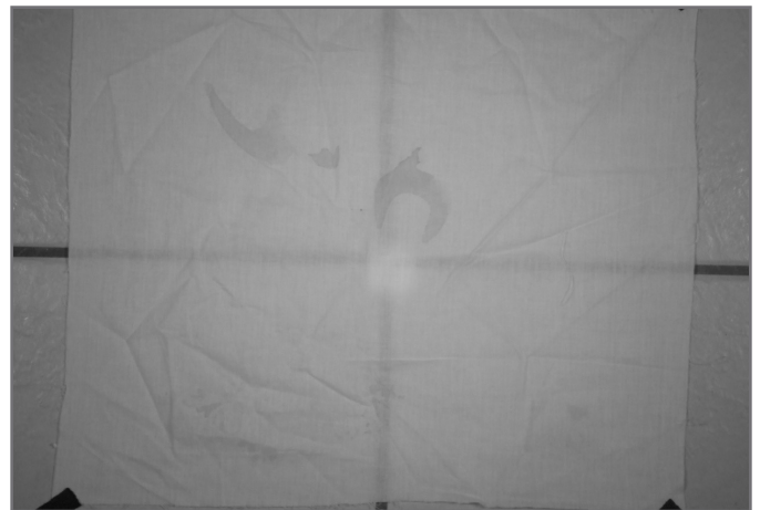
FIGURE 6 The same section of fabric as seen in Figure 5 photographed with a full-spectrum camera equipped with an infrared filter (Wratten 87A equivalent). Illumination was made using photo flood lamps.
