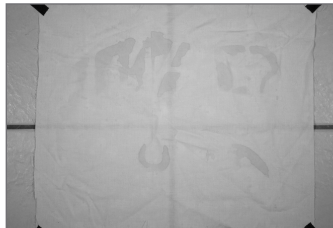
FIGURE 8. The same section of fabric as seen in Figure 7 photographed with a full-spectrum camera equipped with an infrared filter (Wratten 70 equivalent). Illumination was made using photo flood lamps.
