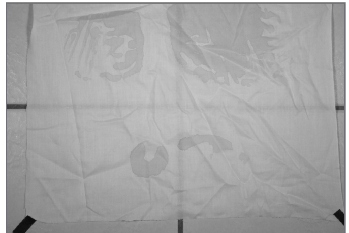
FIGURE 2. The same section of fabric as seen in Figure 1 photographed with a full-spectrum camera equipped with an infrared filter (Wratten 88A equivalent). Illumination was made using photo flood lamps.
