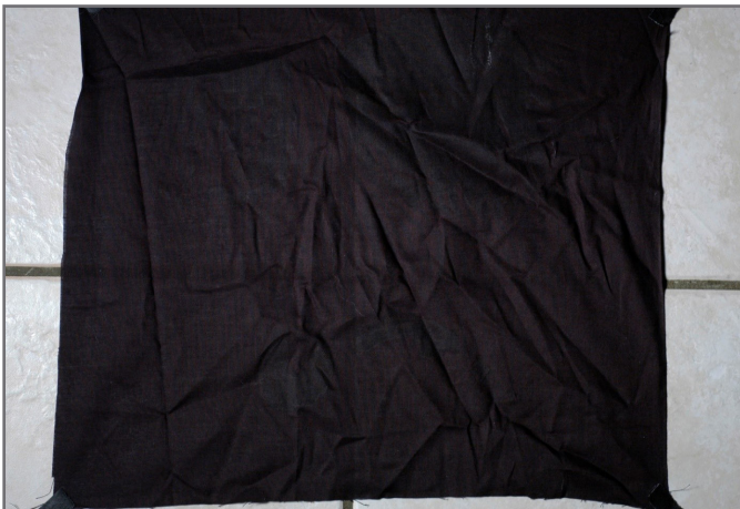
FIGURE 1. Example of a bloodstained section of black fabric photographed with a normal digital camera under visible light.
