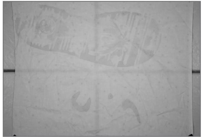
FIGURE 4. The same section of fabric as seen in Figure 3 photographed with a full-spectrum camera equipped with an infrared filter (Wratten 70 equivalent). Illumination was made using photo flood lamps.
